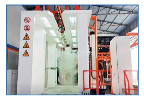
Project name: Fully automatic powder coating line Products: 3D wire mesh fence Product max. size: 3500\*2500\*100mm Design capacity : 1000pcs/10h The space size: L65\*W12m Heating source:LPG
