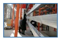
Dip Coating line for fence. The the line is making for dip coating method. Pretreatment will be done separately with a dipping tank. The first step is preheating with 350°C temperature. The coating process is done through a fluidized bed. Then the workpiece moves to curing oven.
