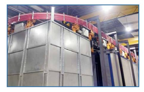
The power and free overhead conveyor system is also called the power and free conveyor. This system can transport and temporarily store workpieces on the conveyor line, to prevent the workpiece from continuing to be transported, and adjust the piece space and movement of workpieces. The items to be transported should not be too small. Gravity roller wheel and rollers are the cheapest and simplest storage conveyors commonly used.
